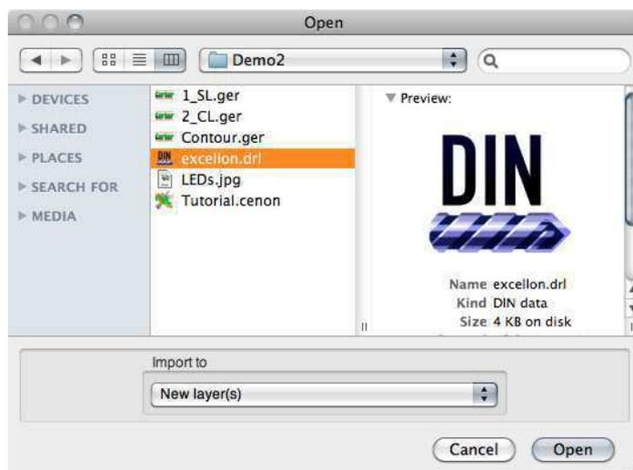
Again it can happen that the drill data is not aligned with the rest of our layout. In the same way as we have learned for the component layer, we can now align the drill data of each drill-layer with the Soldering Layer.
